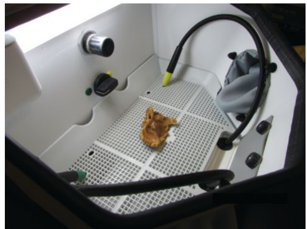
Figure 3. Petrosal portion of temporal bone prior to processing. The Reich Laboratory uses a "sandblaster," pictured here, to extract the cochlea.
